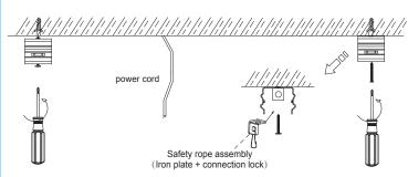
Install the wire safety rope and connect the power cord
